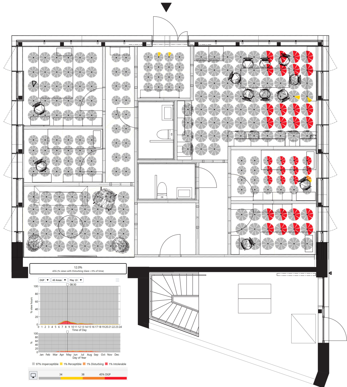
Figure 4.5.5: Daylight Glare Probability (DGP) analysis for the KTH Live-in Lab on May 10th at 8:30 AM. Areas marked in red indicate regions with high glare probability (intolerable glare), while areas in yellow and grey represent perceptible and imperceptible glare levels, respectively. The chart below the floor plan illustrates the percentage of time each glare level is experienced throughout the day. Additionally, the analysis shows that 12.0% of views have disturbing glare for more than 5% of the time (sDG). This analysis helps identify critical areas where glare reduction measures are necessary to improve occupant comfort. Source: Gregor Ruta.
