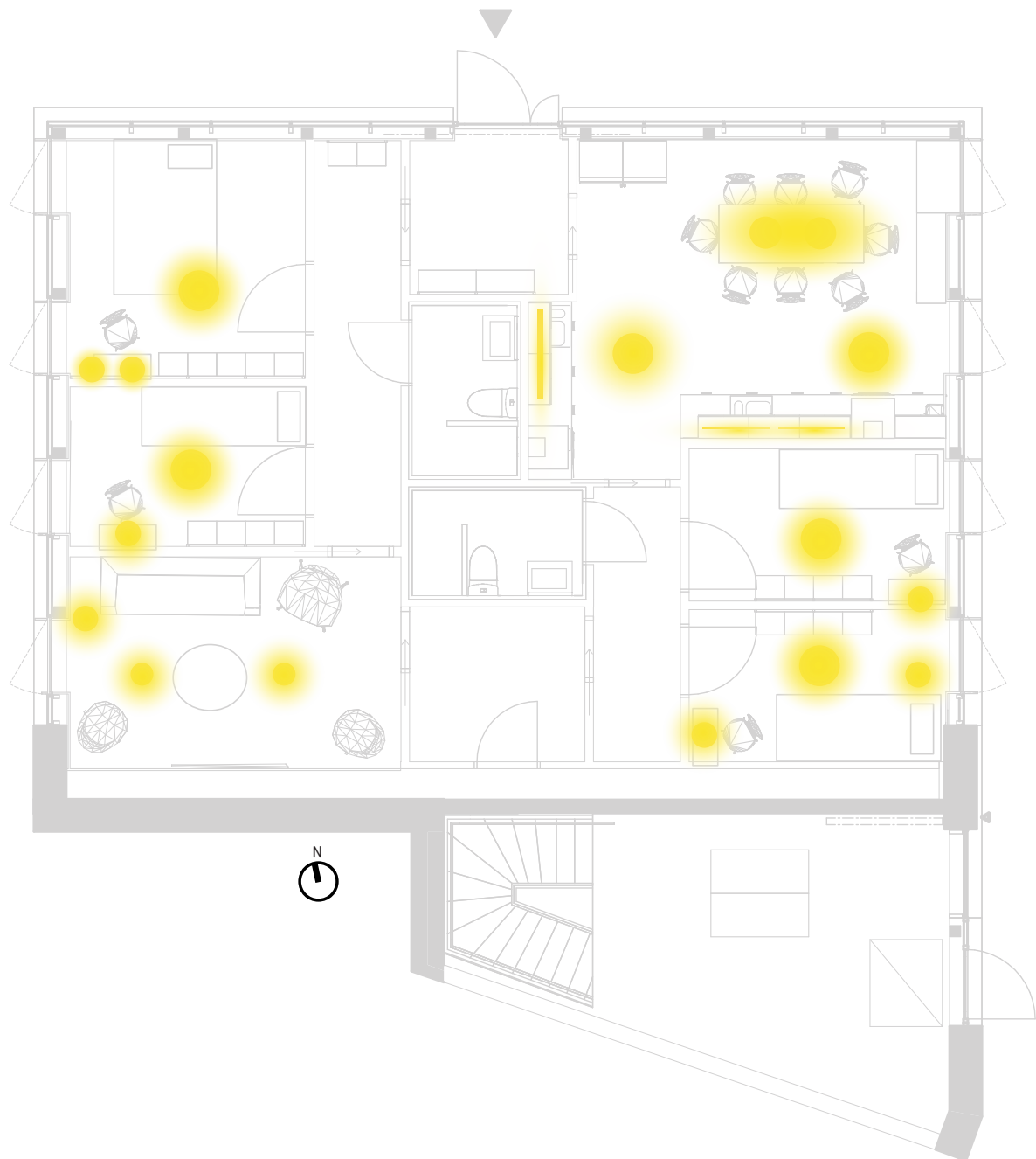
Figure 3.7.1: Lighting fixtures distribution.
