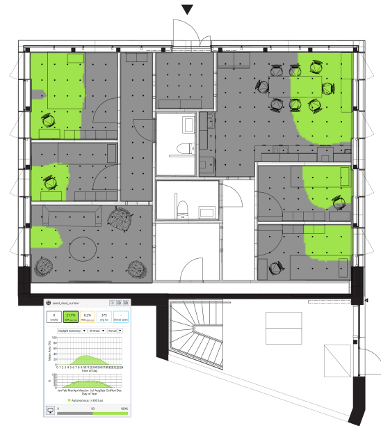
(b) LEED Spatial Daylight Autonomy (sDA) analysis for the dual-section curtain setup, showing an increase to 21.7%. The dual-section design relevantly improves daylight penetration and autonomy.
